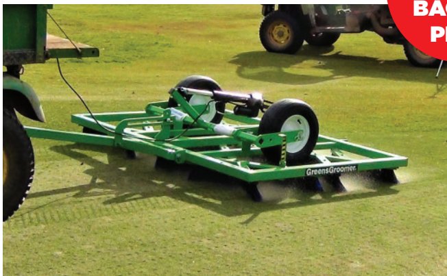
Brushes sand down coring holes
