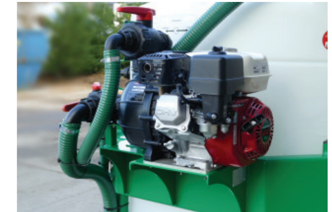
5hp Honda engine with high capacity pump and inline filter unit to prevent blocked nozzles
