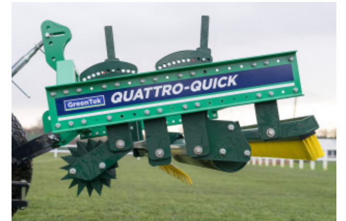
The Spring Rake is adjustable for intensity of grooming and thatch control
