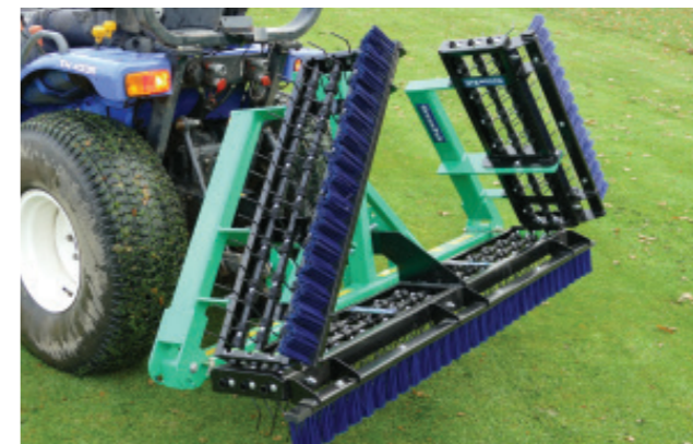
Turf Conditioner 12 with folding wings
