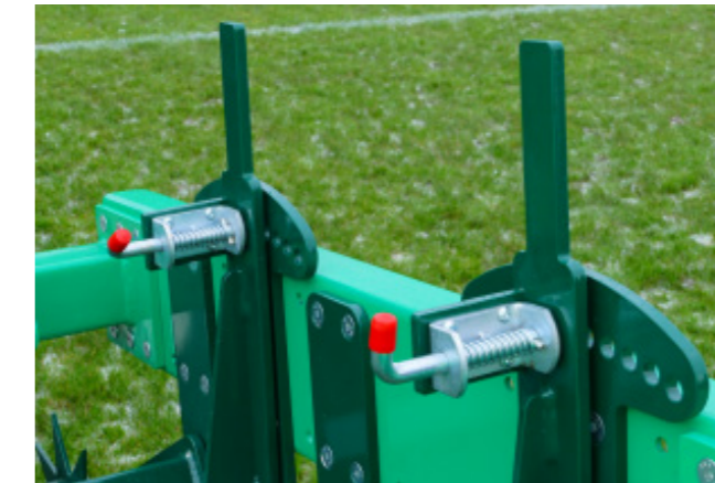
A single lever height adjuster for each implement enables quick and easy set up
