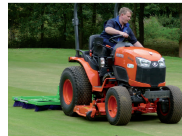
Brushes sand down coring holes
