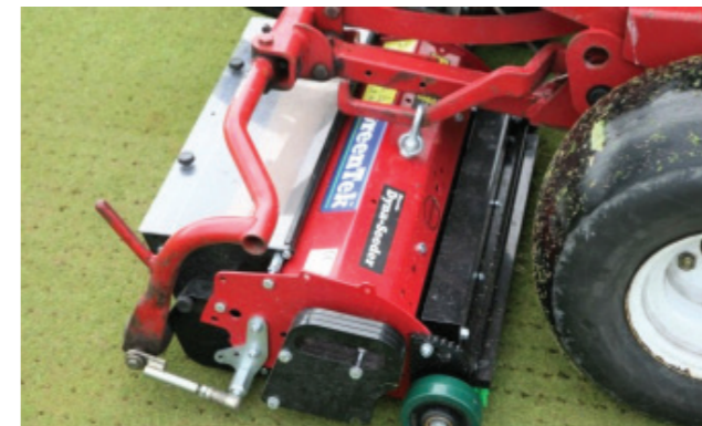
Vibrating spikes create 1,200 holes per square meter for consistent seed distribution.
