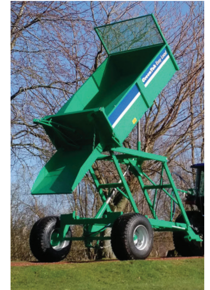
Wheels spaced outside body width provide extra stability for high tipping.
